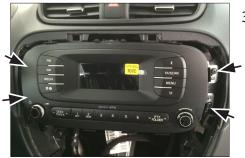
3. Remove all screws of OEM head unit
