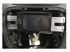
Connect all required circuit points and place double DIN head unit on dashboard. Fix head unit with original screws
